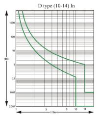
D type protection characteristic curve
