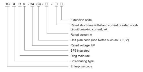
Note: N means non-extension; L means left extension; R means right extension; LR means extension at both sides; C: Load switch unit; F: Combined apparatus unit; V: Circuit breaker unit
