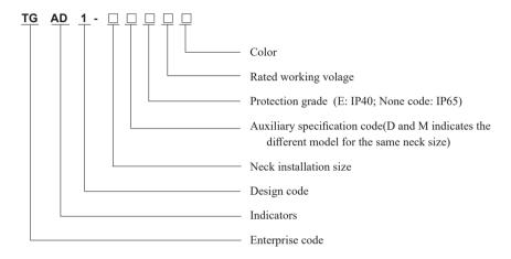
Note: Explanation of auxiliary specification codes (D, M): D indicates an arc round lampshade, and M indicates a buzzer (see Table 1).
