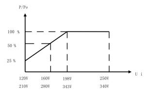
P — Actual output capacity, VA Pe — Rated output capacity, VA Input voltage V Single-phase  $120 \sim 250 \text{V}$  Three-phase  $210 \sim 430 \text{V}$
