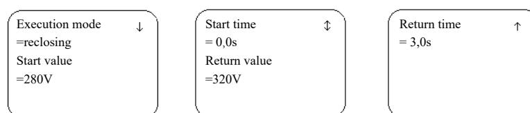
When the measured line voltage is below the start value 280V that is an operating voltage, the controller will issue an opening signal instantly after 0.0s to make the shunt coil or undervoltage release work; when the voltage recovers to the return value 320V, the controller will issue a pulse signal to the closing coil after 3.0s to activate it to conduct the automatic reclosing operation.
