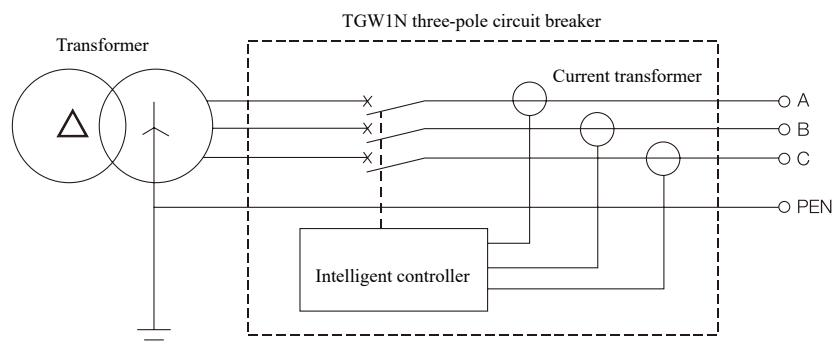
Differential ground fault protection, with the signal from the vector sum of three-phase current (Three-phase unbalance)
