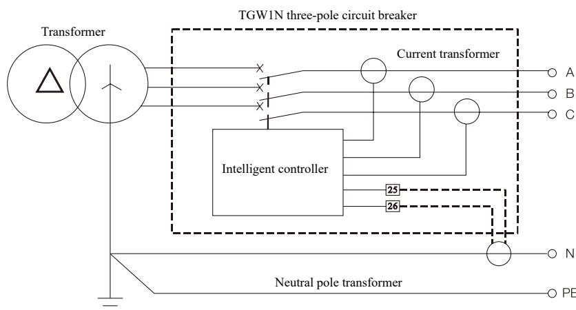
Differential ground fault protection for external neutral pole transformer, with the signal from the vector sum of three-phase current and N pole current only
