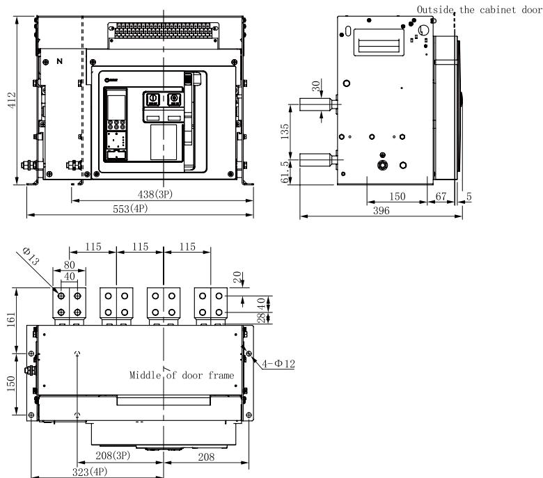
11.13 Outline dimension and installation dimension drawing of TGW1N-4000 (In=3600-4000A) drawer type circuit breaker
