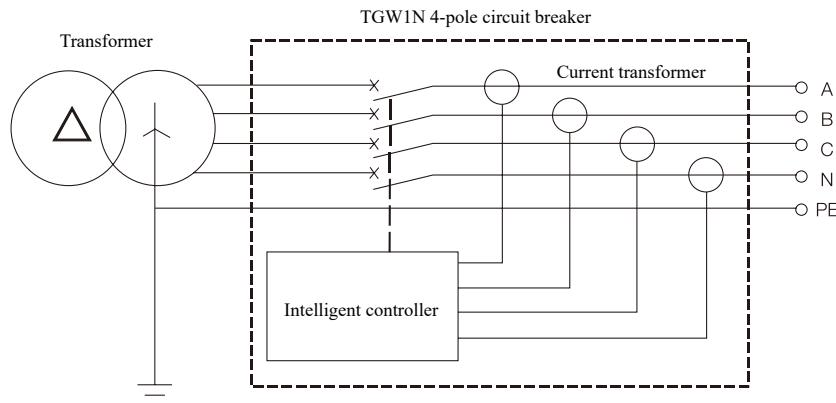
Differential ground fault protection, with the signal from the vector sum of three-phase current and N pole current
