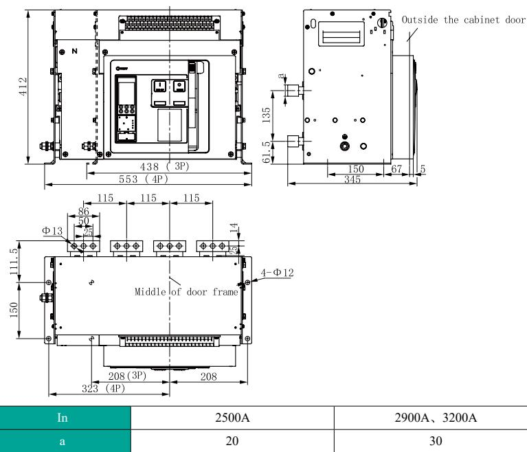
**11.11 Outline dimension and installation dimension drawing of TGW1N-4000( $In=2500\text{-}3200\text{A}$ ) drawer type circuit breaker**
