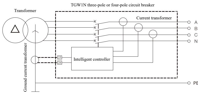
Ground current type ground fault protection of the external grounding current transformer, with the signal between the neutral point of the main power supply and ground.
