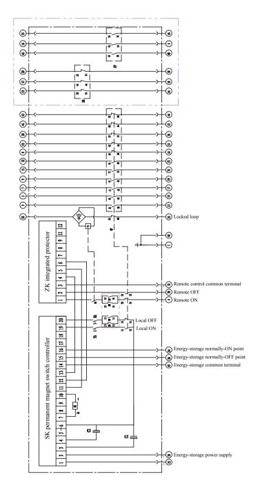
Note: Handcart type is marked with double dots line. No this connector is required for fixed type; 2.5mm² is available for 25# and 35# lines.
