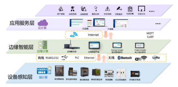
The company's Tianzheng Tianzhi "TenEdge" intelligent power distribution system is based on the Internet of Things architecture, relying on built-in intelligent circuit breakers, modules, etc.
